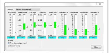
The MeterLink Baseline Viewer™, available in CFA-equipped 3410 electronics, enables operators to quickly confirm the meter is operating within established ranges.
