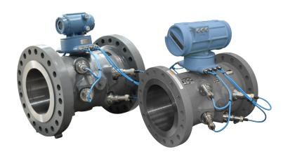
The more compact electronics enclosure is the standard for all Daniel gas and liquid ultrasonic meters. The larger, retrofit electronics enclosure is currently an option for Daniel gas ultrasonic meters only (no optional display available).
