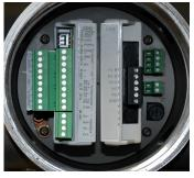
The electronics within the standard enclosure feature a plug-in CPU and I/O module that increases reliability and facilitates expansion.
